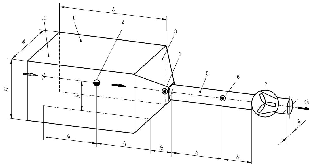
$$\begin{aligned} W/H &\geq 0.66, & l_1 &\geq 0.5 \sqrt{A_c}, & l_3 &\geq 5d; \\ W/H &\leq 1.5, & l_1 &\leq 2.0 \sqrt{A_c}, & l_4 &\geq 3d; \\ h &\leq 0.66H, & l_1 &\leq 2.0 \text{ m}; \\ l_0 &\geq 0.5 \sqrt{A_c}, & 0.5 \sqrt{A_c} &\leq l_2 \leq \sqrt{A_c}. \end{aligned}$$
